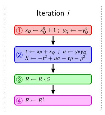
► Sequential dependencies between the tasks in each iteration
