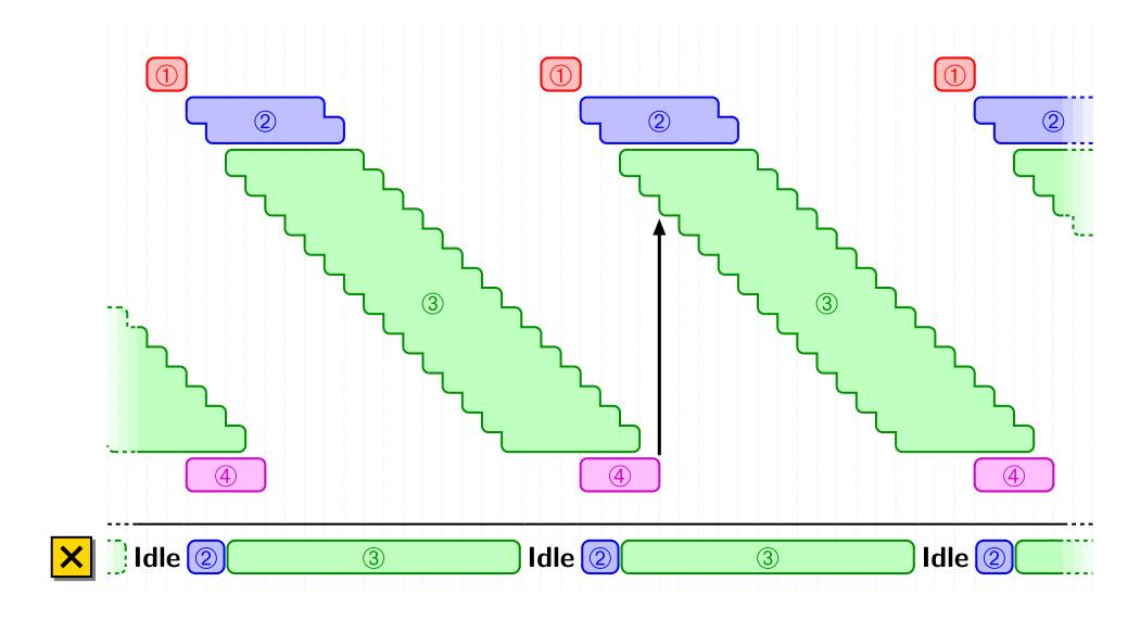
ightharpoonup The task dependency 4 o 3 forces idle cycles into the multiplier pipeline
