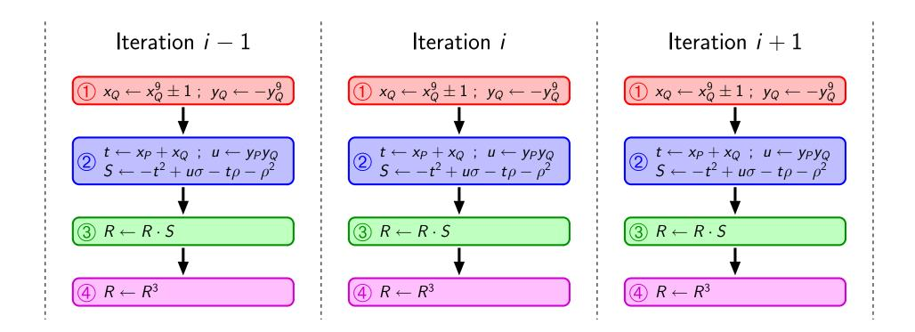
Sequential dependencies between the tasks in each iteration
